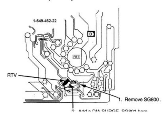
Original Design: SG800 is connected to circuit ground.
